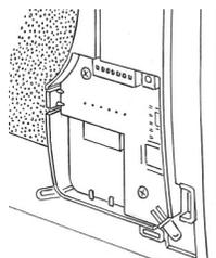
Reinsert the function board with the FM-EO radio module plugged on into the receptacle in the filter frame and screw tight. Insert the antenna of the radio module into the groove of the filter frame provided for this purpose.
