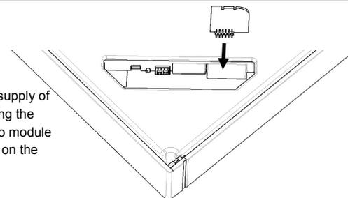
Disconnect the power supply of the Ne<sup>xt</sup> before inserting the module. Insert the radio module into the larger opening on the right as shown.
